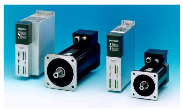
Components of the MaxiDrive servo drives family – at the left: BN 6725 servo amplifier (20 A) with MR 4416 motor (18 Nm at 3000 r.p.m.), at the right: BN 6723 servo amplifier (8 A) with MR 4206 motor (2.8 Nm at 6000 r.p.m.)
