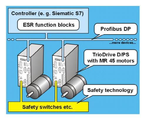
At the SPS/IPC/DRIVES servo specialist ESR Pollmeier presents TrioDrive D/PS, the refined development of its successful digital servo drives. The 230 V servo controller with integrated safety system has been optimized for the use with Profibus DP and comes with increased processor power at a reduced price. Together with the new MR 45 servo motor series, ESR offers the complete servo drive in the torque range from 0.3 to 5 Nm.
